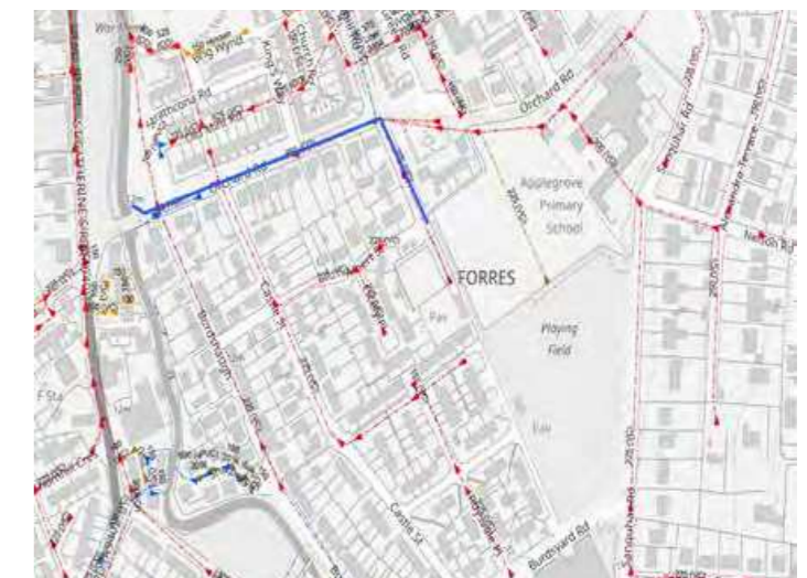
Figure 11. Potential surface water sewer along Orchard Road
