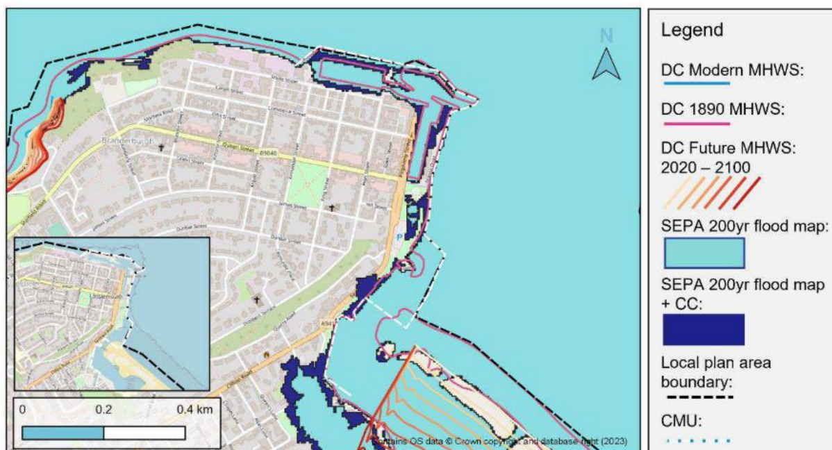
Figure A-9: CMU 3: Harbour town central defended coastal hazards map showing SEPA flooding and Dynamic Coast (DC) past and future erosion. Inset shows CMU without coastal hazards.
