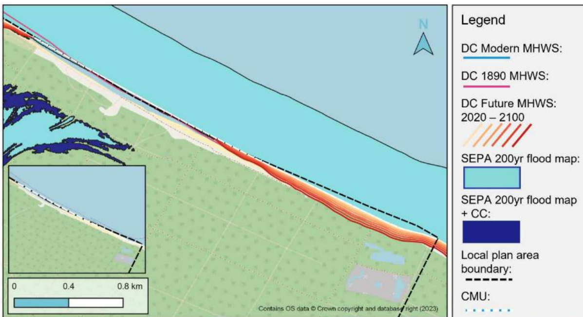
Figure A-15: CMU 6: Shingle beach east natural coastal hazards map showing SEPA flooding extents and Dynamic Coast (DC) past and future erosion. Inset shows CMU without coastal hazards.
