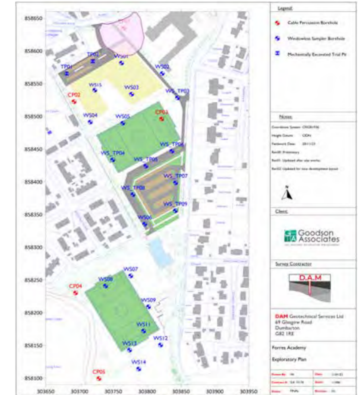
Figure 9. Exploratory plan with area of loose ground highlighted in a pink hatch
