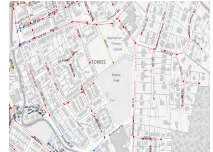
Figure 10. Existing surface water and foul water (combined) system as displayed on Scottish Water maps.
