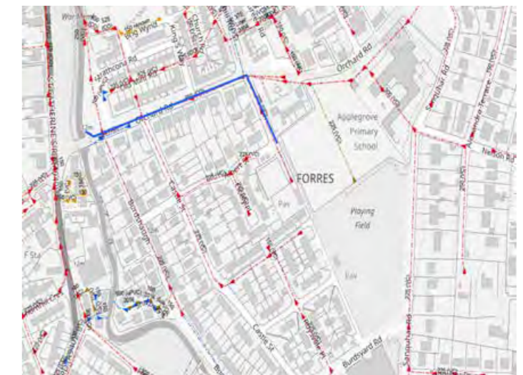
Figure 11. Potential surface water sewer along Orchard Road
