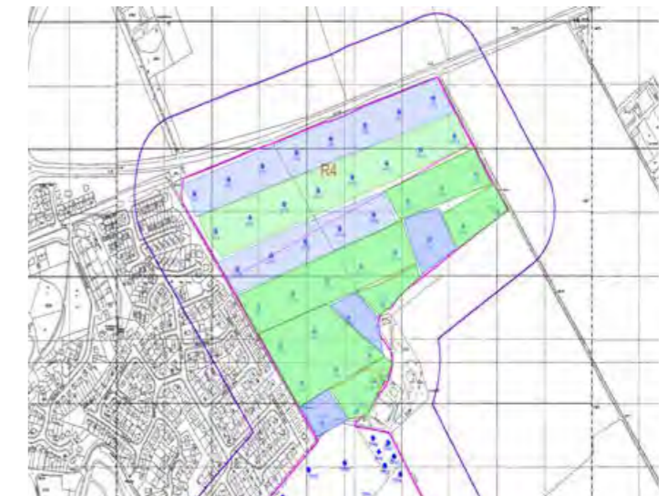
Figure 4. The distribution between loose and medium dense sand. Blue hatch displays trial holes with loose sand present to approximately 1.2-2mbgl. Green hatch highlights holes with loose sand present from approximately 0-1.2mbgl.
