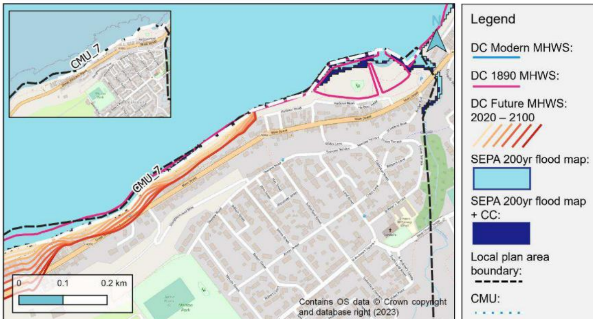
Figure A-13: CMU 6 defended east coastal hazards map showing SEPA flooding extents and Dynamic Coast 2 past and future erosion. Inset shows unit without coastal hazards.
