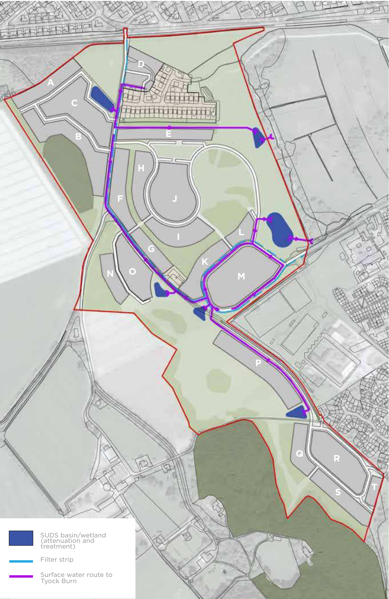
fig. 28: Surface water drainage strategy
