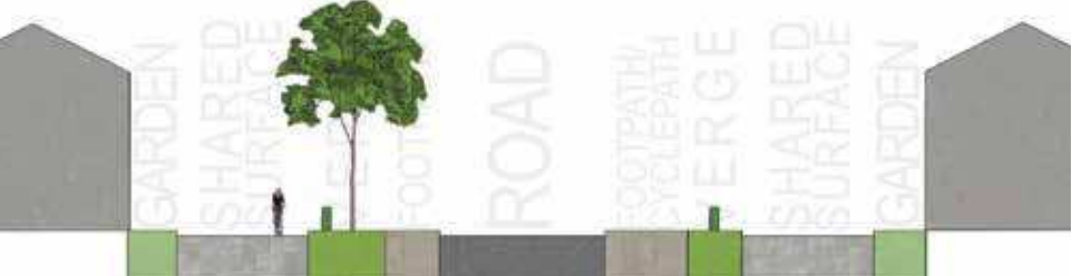
fig. 22: Typical primary street corridor where existing hedgerows are to be retained (Option 2)
