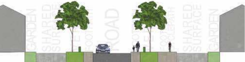
fig. 21: Typical primary street corridor where existing hedgerows are to be retained (Option 1)
