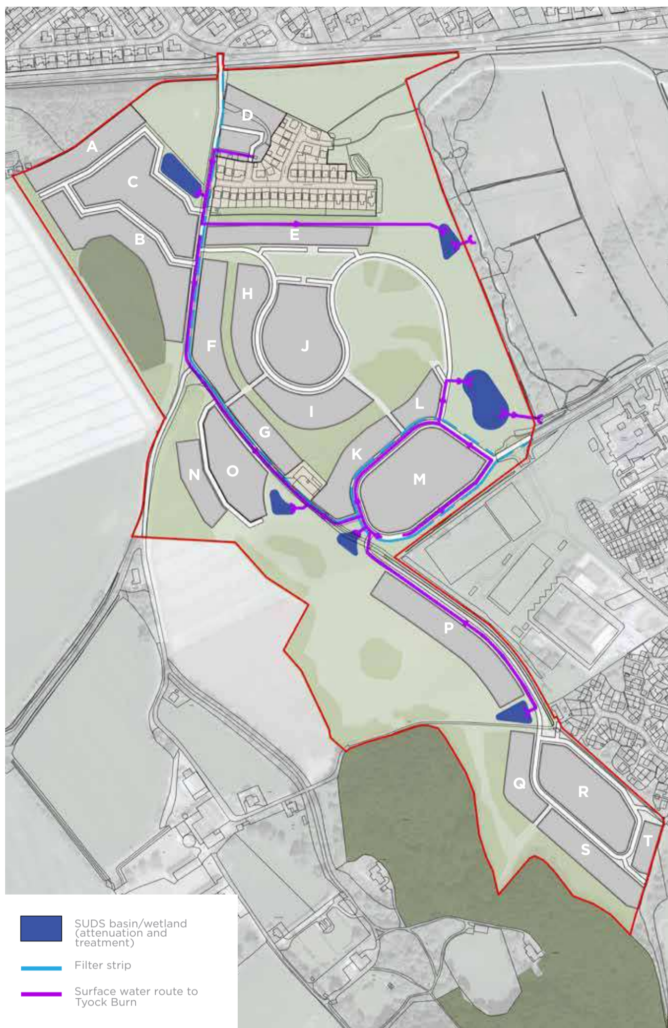
fig. 28: Surface water drainage strategy
