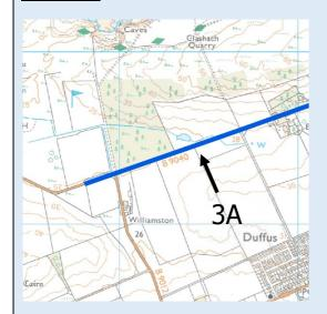
Section 3A would run within the verge on either side of the road eastbound as a continuation of the existing cycleway. East of the B9012 the existing verge narrows to around 1.5m on both sides of the carriageway and third party land would be required for either a northern or southern alignment with the cycleway provided adjacent to the carriageway.
