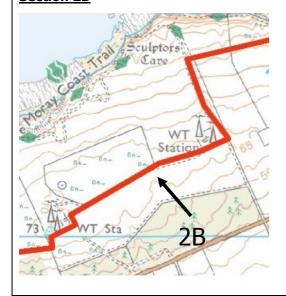
Section 2B would utilise the existing tarmac surfaced road running on a level gradient for 700m past the radar station. At the end of the tarmac surface it is assumed that the route would require to turn left and proceed downhill on a 7% gradient to avoid bisecting existing agricultural fields. At the field boundary the route would turn right and proceed east.
