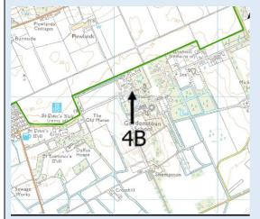
The alternative alignment for section 4B would turn south along the western edge of Duffus before following the outer boundary of the adjacent field to the east before turning to the north and then east, continuing along the northern boundary wall of Gordonstoun. An alignment through this section would minimise the number of filed crossings although would add an further 600m compared to the option described above.
