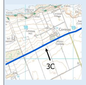
A southern alignment would run within the existing field boundary around 4m from the carriageway edge to account for the change in level between the carriageway and adjacent field which will result in additional land take. A northern alignment would run adjacent to the carriageway although a diversion would be required at Wester Covesea Farm and a single residential property to the west due to lack of available verge width.
