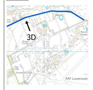
Section 3D would continue along the B9040 either to the north of south of the carriageway. North of the carriageway a number of access crossings would be required and is recommended that the preferred alignment would be to the south of the carriageway east of the Lossie Equestrian Centre to take advantage of increased verge width and the limited alignment option from North Greens to Lossiemouth.
