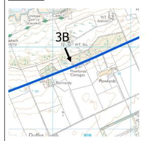
Due to the available verge widths between a number of properties and the carriageway through Section 3B it will not be possible to deliver the route alongside the B9040 and a diversion will be required to pass Burnside Farm and Pewlands Cottages to the south or Burnside House and two further residential properties to the north.
